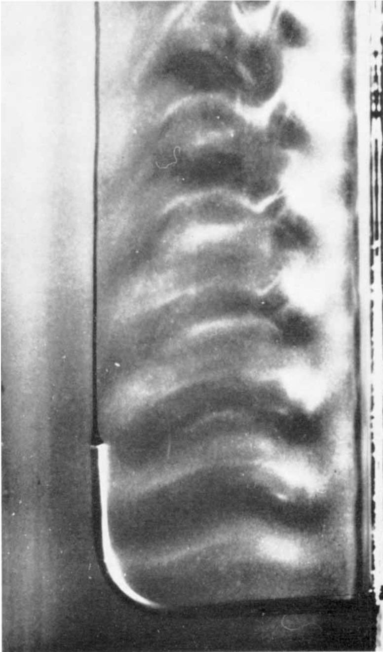
FIGURE 1. Wake of a 0.048 in. diameter probe in the laminar flow of a birefringent liquid, showing a stable dye trace and a disturbed birefringent pattern.
